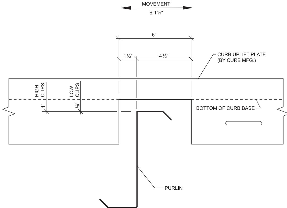
UPLIFT PLATE MUST BE FIELD NOTCHED AROUND THE BUILDING PURLIN TO ALLOW FOR PANEL MOVEMENT.
