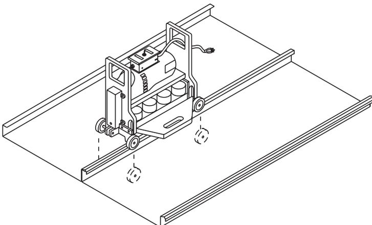
Stop seamer about one foot from end of panels. Disengage locking bar and remove the electric seamer. Finish seam with hand tool.
