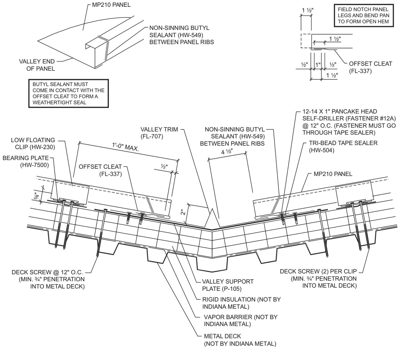
**NOTE: DO NOT USE THIS DETAIL ON ROOF SLOPES LESS THAN 3:12**
