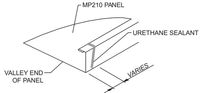
URETHANE SEALANT MUST COME IN CONTACT WITH TAPE SEALER TO FORM A WEATHERTIGHT SEAL
