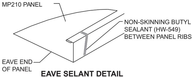
BUTYL SEALANT MUST COME IN CONTACT WITH THE DRIP EDGE TO FORM A WEATHERTIGHT SEAL
