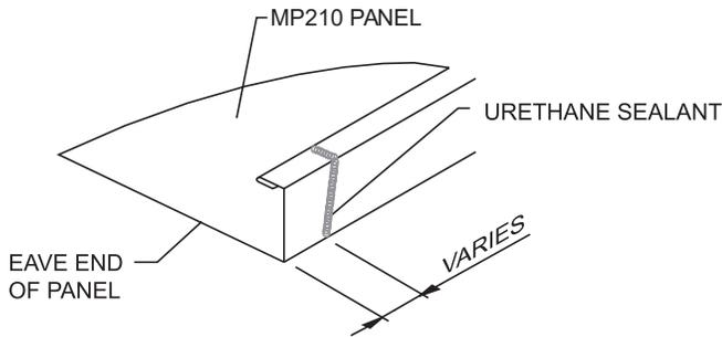
URETHANE SEALANT MUST COME IN CONTACT WITH TAPE SEALER TO FORM A WEATHERTIGHT SEAL
