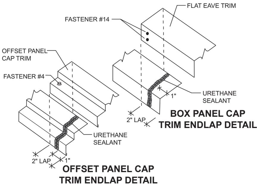
Lap trim 2". Apply two beads of urethane sealant between the trim pieces, approximately 1" from the end of the bottom piece. Attach trim laps in flat eave trim with Fastener #14. Attach trim laps on panel cap trim with Fastener #4.
