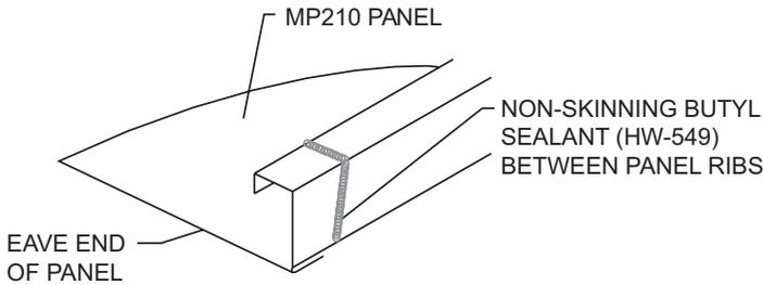
BUTYL SEALANT MUST COME IN CONTACT WITH THE DRIP EDGE TO FORM A WEATHERTIGHT SEAL
