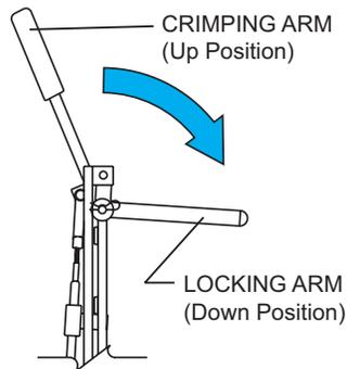
Push locking arm down to lock crimper onto seam. If difficulty is encountered, check to make sure that the hand crimper is properly aligned on seam. **Do not force locking arm.**
