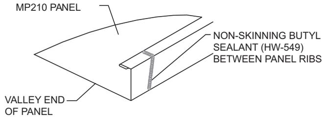
BUTYL SEALANT MUST COME IN CONTACT WITH THE OFFSET CLEAT TO FORM A WEATHERTIGHT SEAL
