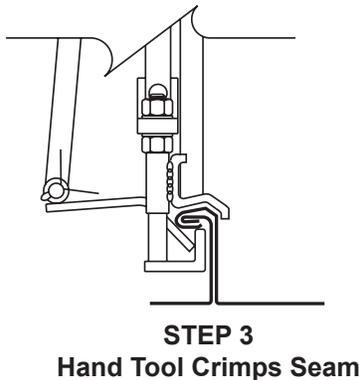
Push crimping arm down to crimp panel. Return both the crimping arm and locking arm to the up position and remove tool from seam.
