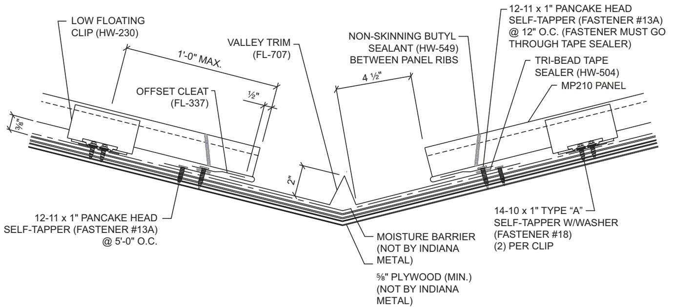
NOTE: DO NOT USE THIS DETAIL ON ROOF SLOPES LESS THAN 3:12
