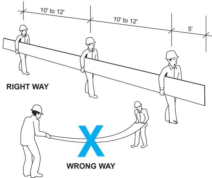
Standing on one side of the panel, lift it by the seam. If the panel is over 10' long, lift it with two or more people on one side of the panel to prevent buckling.
