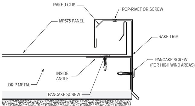
1. Install the continuous rake j-clip to the decking before installing panels using pancake screws, 30" max O.C.
