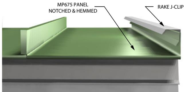
2. If roof requires a partial panel, measure width and add 1", then use a folding tool to bend a 90° leg.
