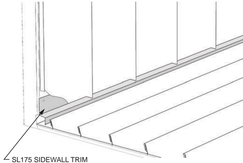
Overlap the trims by 3" using a bead of sealant between laps
