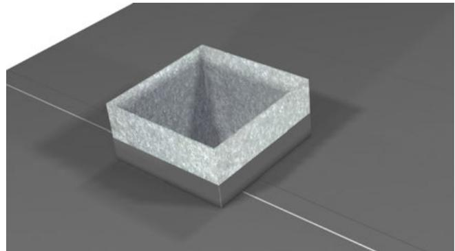
2. Fit angle flashing to the square protrusion. Flashing should be a minimum of 4" x 4". Bend tabs around box; fit lower flashing first, then fit side flashings, followed by upper flashing tabbed over the side flashings. Caulk all joints and fasten with recommended clip screws.
