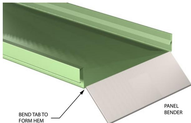
Step 3: With the hemming tool bend the tab down and under to form a 180° bend.
