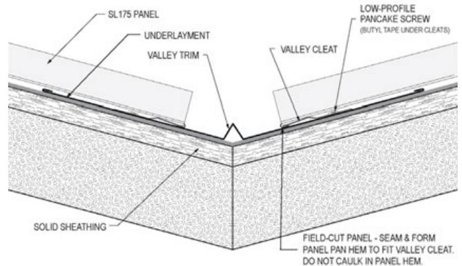
4. Fabricate an open hem on each panel at the correct pitch for the valley. Slide the panel up to engage the cleat, snap in the panel at the rib, and screw male side of panel to decking.
