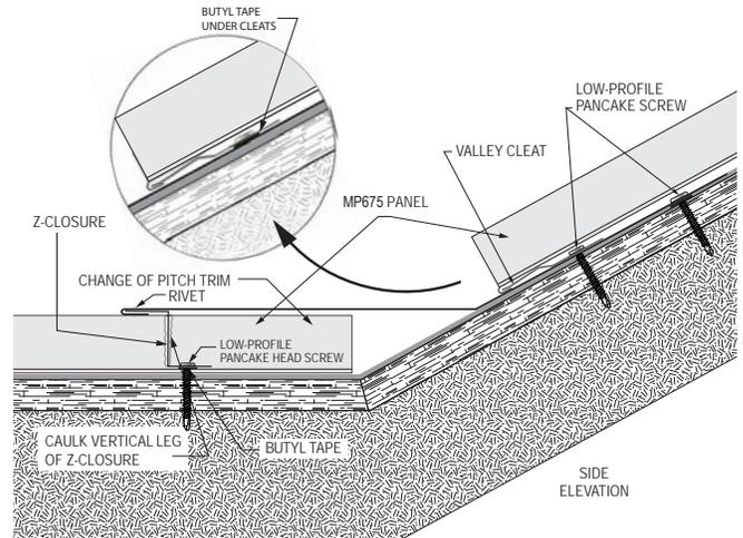
3. Install cleats 4"- 5" up from the center of Change Of Pitch trim using low-profile pancake screws and sealant. Seal the cleat to the trim using butyl tape or caulk. Apply panels to upper roof overlapping COP transition by 5".
