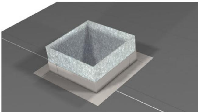
3. Cover angle flashing with a second layer of underlayment to protect against metal-to-metal contact.
