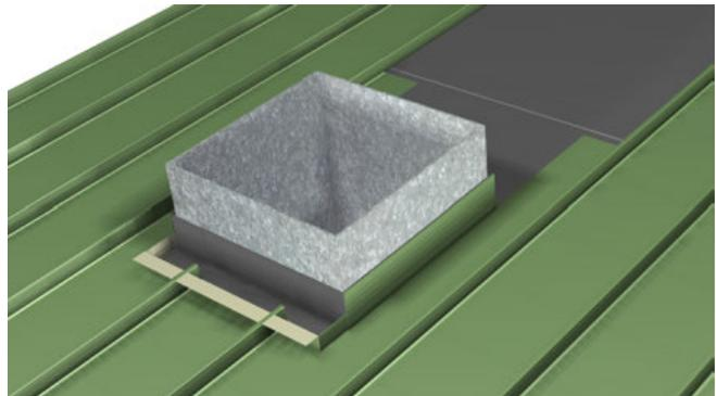
6. Attach the roof to wall flashing and caulk all joints. Use rivets to attach the z-closure. Caulk z-closures as typical, and rivet flashing at overlaps.
