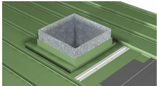
11. Fit and hem roof panels above the penetration. Clip panels onto the cleat. Do NOT caulk between panel and cleat.
