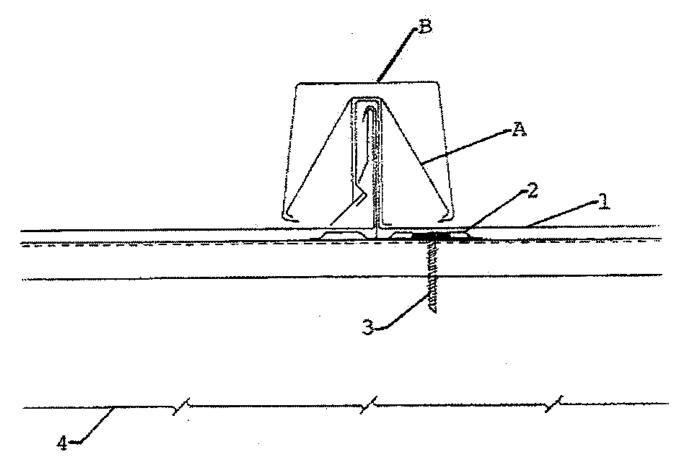
1. Metal Roof Deck Panels\* — No. 24 MSG min thickness coated steel. Panel width 18 in. max., 10 in. min. Rib height 1-3/4 in. at female side. Panels continuous over two or more spans. A bead of sealant may be used at panel side joints.
