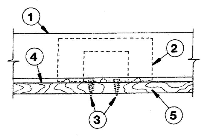
1. Metal Roof Deck Panels\* — No. 24 MSG min coated steel. Panel width 18 in. max., 10 in. min. Rib height 1-3/4 in. at female side. Panels continuous over three or more clips with no endlaps. A bead of sealant may be used at panel side joints.
