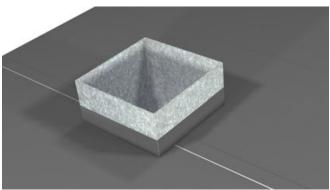
Fit angle flashing to the square protrusion. Flashing should be a minimum of 4" x 4". Bend tabs around box; fit lower flashing first, then fit side flashings, followed by upper flashing tabbed over the side flashings. Caulk all joints and fasten with recommended clip screws.
