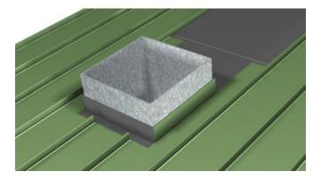
Align the counter flashing and z-closure, marking the z-closure location. Apply butyl tape to the z-closure, and fasten the z-closure with clip screws. Fold tabs from the z-closure back to the sides of the protrusion. Install the roof to wall counter flashing.
