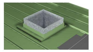
10. Run butyl tape and attach cleat to roof approximately 10" above the penetration, on top of the flashing. Fasten with clip screws every 12 inches.
