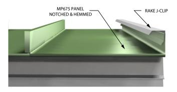
2. If roof requires a partial panel, measure width and add 1", then use a folding tool to bend a 90° leg.
