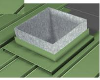
8. Fit & tab upper (ridge-side) angle flashing. Flashing base should be a minimum width (see table below) to accommodate cleats and roofing panel joint.
