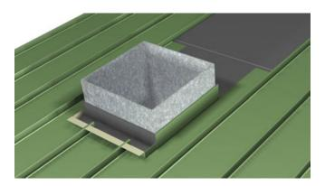
Attach the roof to wall flashing and caulk all joints. Use rivets to attach the z-closure. Caulk z-closures as typical, and rivet flashing at overlaps.
