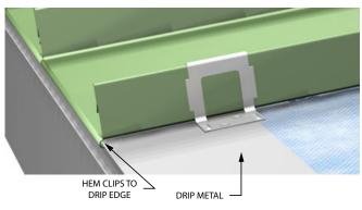
5. Leave a tab when notching the rib, and use sealant in panel ends. Fold over the tab end of the rib for a more finished look.
