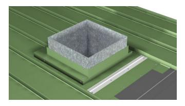
Fit and hem roof panels above the penetration. Clip panels onto the cleat. Do NOT caulk between panel and cleat.
