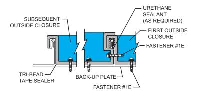
Use urethane sealant to fill any voids around the panel seams on the upslope side of the outside closures.
