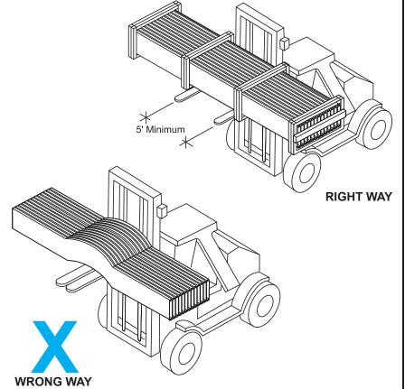
When lifting bundles with a forklift, forks must be a minimum of five feet apart. Do not transport open bundles. Drive slowly when crossing rough terrain to prevent panel buckling.
