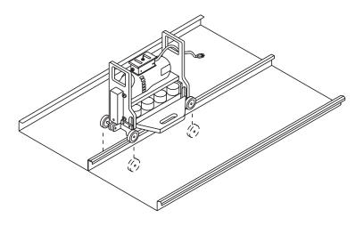
Stop seamer about one foot from end of panels. Disengage locking bar and remove the electric seamer. Finish seam with hand tool.
