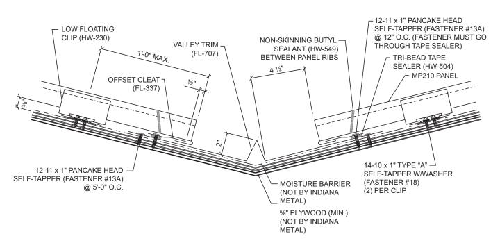
NOTE: DO NOT USE THIS DETAIL ON ROOF SLOPES LESS THAN 3:12
