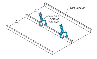
Clamp the panel seam together at both ends. Long panels may require one or more clamps in the middle. This will help hold panel module.
