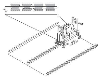
To begin seaming, set seamer on seam with the locking bar up and to the open side of the seam. The rear wheels should be even with the edge of the roof panel. Push the locking bar down to engage the rolls and turn the seamer on.
