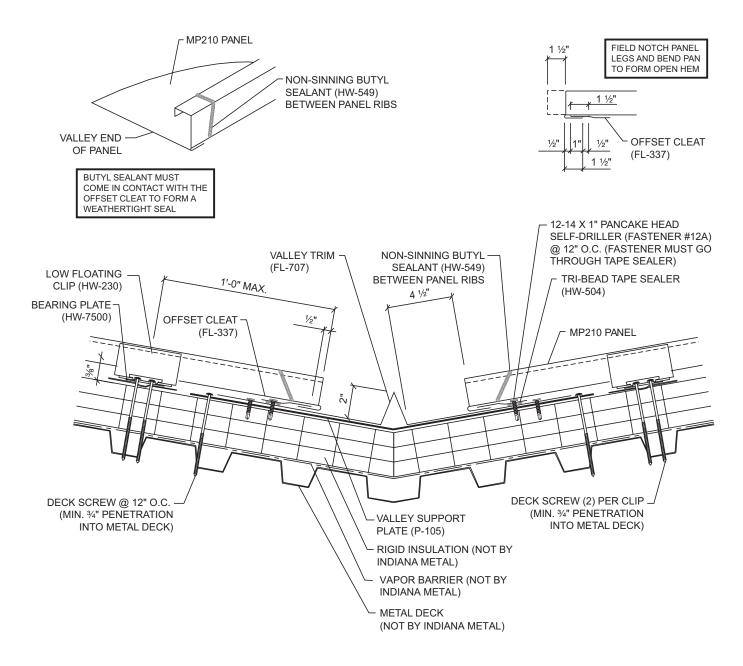
NOTE: DO NOT USE THIS DETAIL ON ROOF SLOPES LESS THAN 3:12
