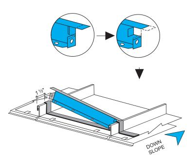
Field cut the end of the outside closure that fits to the open side of the panel seam. Notch and bend the vertical leg of the closure above the end tab back to the dimple formed into the closure. It is important that the closures fit tight to the panel seams to prevent the need for excess urethane sealant at this location.
