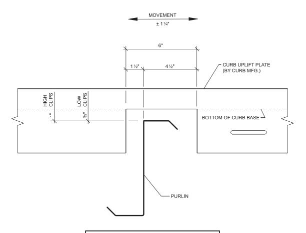
UPLIFT PLATE MUST BE FIELD NOTCHED AROUND THE BUILDING PURLIN TO ALLOW FOR PANEL MOVEMENT.
